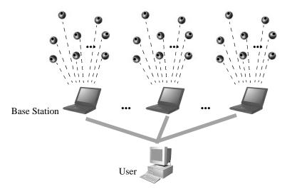
Figure 1: This figure shows an example sensor network with small video sensor devices that are inexpensive to build and have limited capacity to forward data to a base station which serves as an aggregator of data. Users access these base stations for information that they require.
