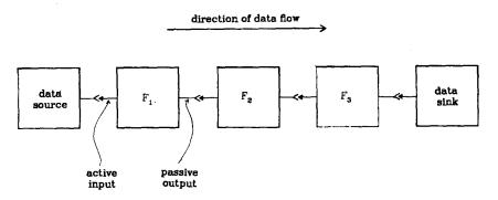
Each box represents an Eject. The filters  $F_i$  all perform active input and passive output. The sink actively inputs and the source passively outputs.
