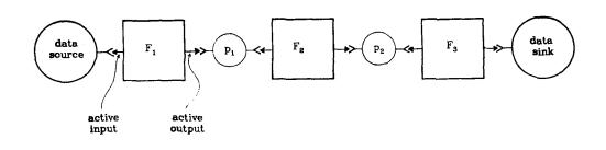
$F_1$ ,  $F_g$  and  $F_3$  are filters. The shape of the connectors on the filters indicate that they are performing active input and active output. The circles represent facilities provided by the Unix kernel.  $p_1$  and  $p_g$  are pipes; data source and data sink may be files or devices.
