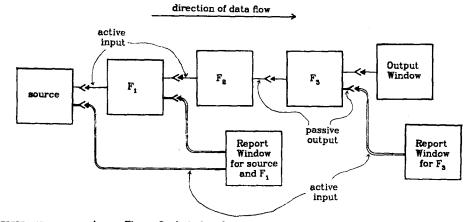
The same arrangement as Figure 3, but in the "read only" discipline. The double lines indicate *Read(ReportStream)* requests; the single lines indicate *Read(Output)* requests. It is assumed that the Report Window is designed to read from multiple sources.
