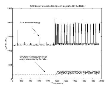
Figure 2: Sample energy trace: note simultaneous measurement of radio and system-level energy cost.
