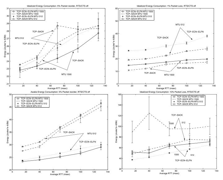
Figure 5: Idealized and awake energy for 5% packet reordering.
