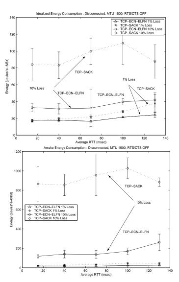
Figure 4: Idealized and awake energy cost for the route failure case.
