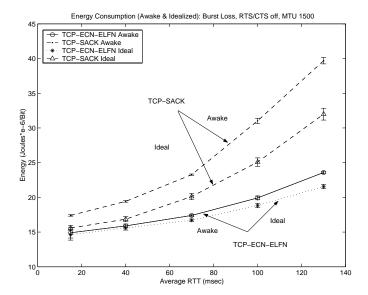
Figure 7: Energy for bursty losses.
