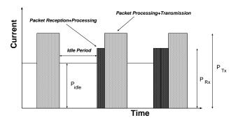
Figure 1: Simplified energy consumption profile.
