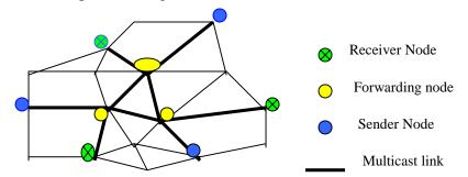
The key features of FG infrastructure are reduced storage overhead, allows loose connectivity among multicast group members, which makes protocol more scalable for large networks and more stable for mobile wireless networks.
