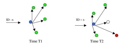
[At time T2 a copy of same packet x arrives, and in the mean time host (blue) has got new neighbor (red) so if host does the rebroadcast then other nodes (green) will have unnecessary broadcast (at least four), to avoid this superfluous broadcast the host can inform that it is re-broadcast for new neighbor (red)]
