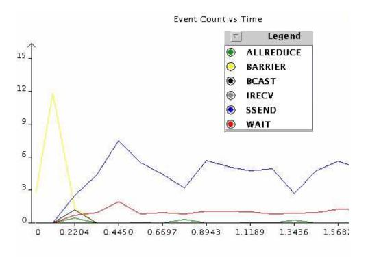
Figure 14: Histogram of MPI Constructs in su3\_rmd
