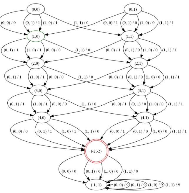
This is exactly analagous to the Ripple Carry Adder
