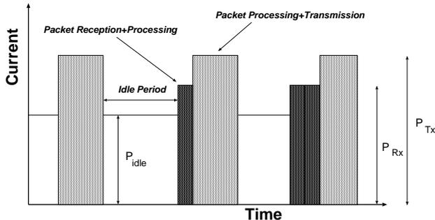
Figure 1: Simplified energy consumption profile.
