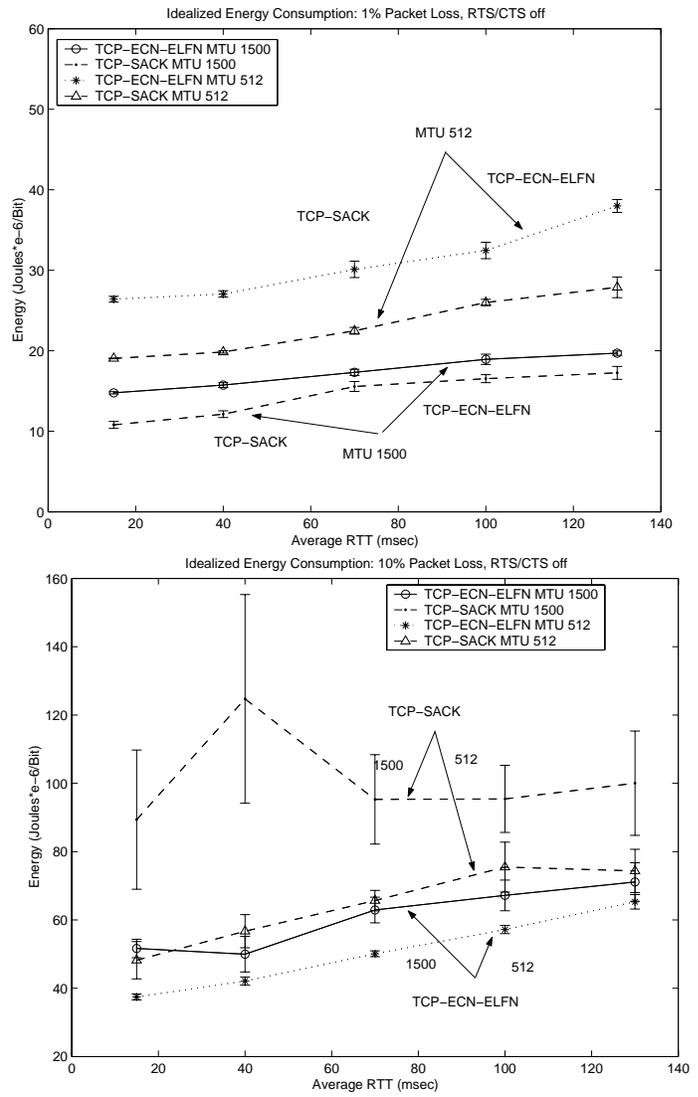
Figure 6: Idealized energy cost for loss case.
