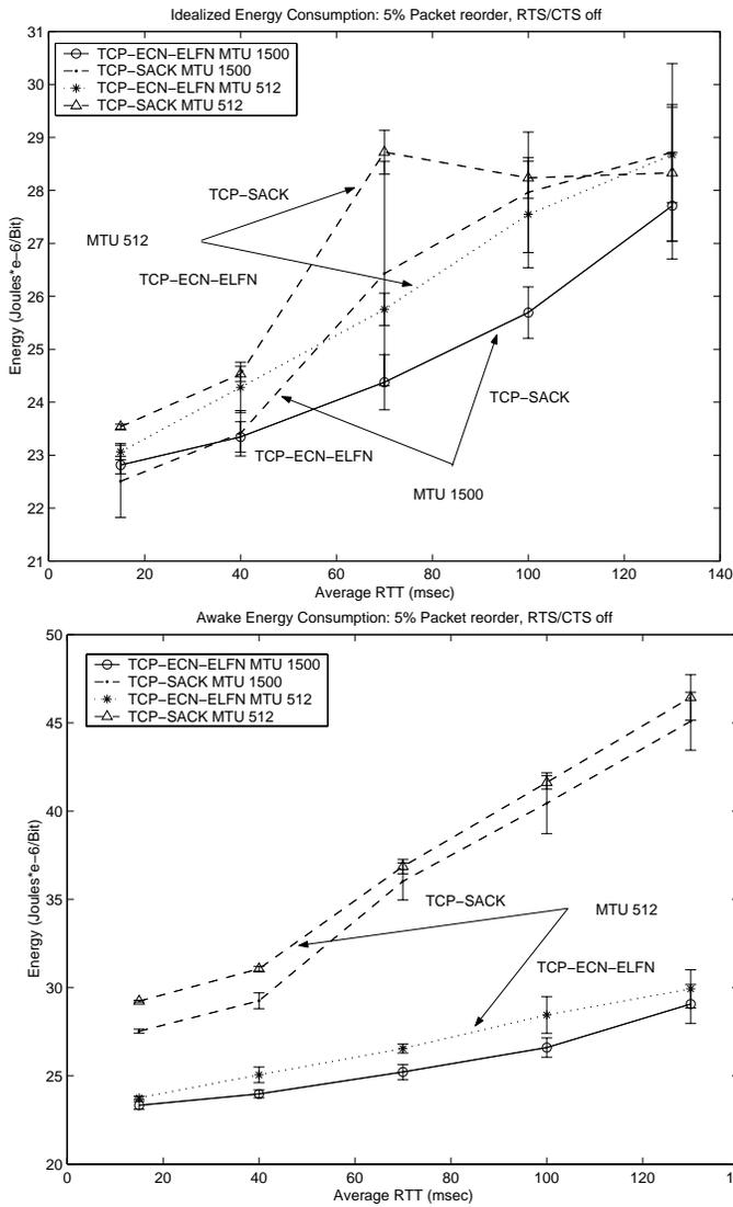
Figure 5: Idealized and awake energy for 5% packet reordering.
