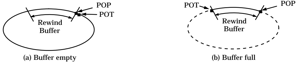
Figure 4.4: Buffer Limit Conditions. Figures (a) and (b) show the cases that occur during playback when the buffer is empty and full, respectively. The solid line represents data that has been played back but not removed from the buffer, while the dashed line represents data that has been transmitted but not played back.
